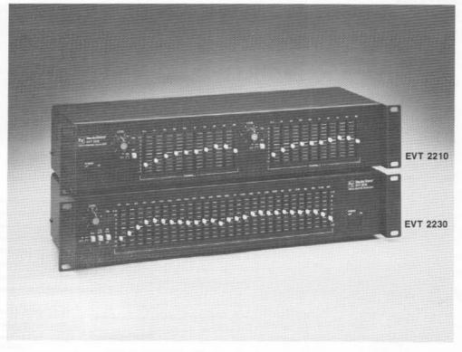
The true combining filter design of the EVT 2230 results in smoother phase and frequency response, especially between bands. An EQ in/out switch is provided so that the equalizer and filter portions of the unit may be bypassed, allowing for instant comparison of equalized and unequalized settings. Peak responding level dectors are used and the LED's on time is increased by a peak stretching circuit, so that even very short overload transients are visually
