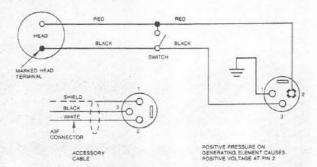
FIGURE 2 — Wiring Diagram
