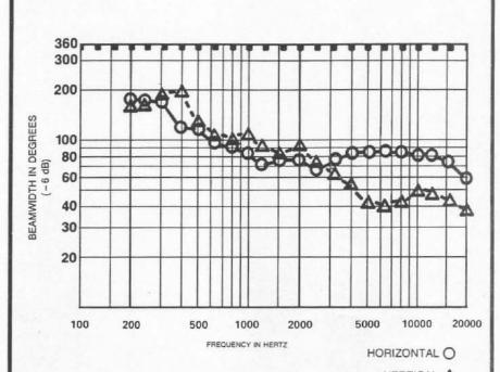
FIGURE 4 — Beamwidth vs Frequency
