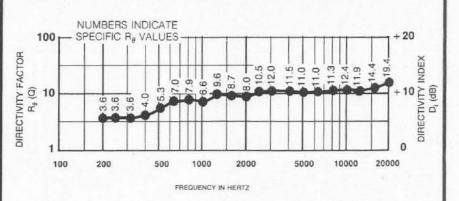
FIGURE 5 — Directivity vs Frequency Whole Space (anechoic)
