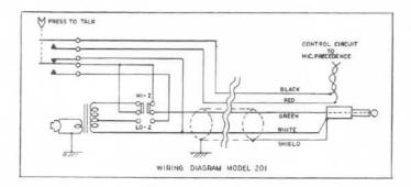
If more than one microphone is to be used to mute the music while paging, connect the control wires from these microphones IN PARALLEL across the microphone precedence terminals on the Raymer unit.
