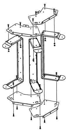
FIGURE 6 — Installing System 200™ Speakers into the Mb200 Brackets (exploded view)
