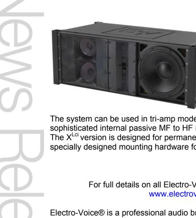
The EV X<sup>LC</sup> 127 is a 3way design that utilizes a 12" vented LF, 2 x 6.5" MF transducers on a 120degree horizontal waveguide, and 2 x HF transducers that combine through a new vertical plan wave generator to a 120-degree waveguide.
