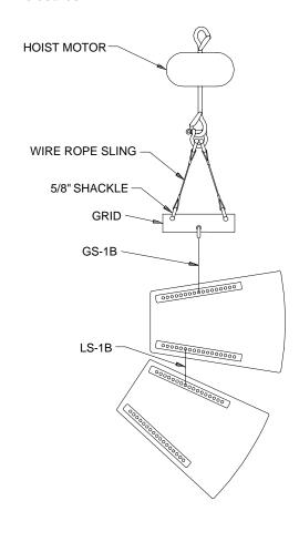
Figure 2.2—Xi Dimensions, Weight, Rigging Location and Center of Gravity
