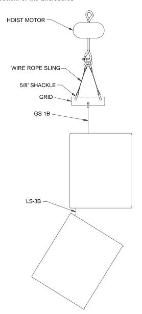
Figure 2.1b—Rigging Hardware on the Sides of the Enclosures
