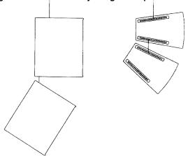
from one another (an Xi-1122 suspended beneath an Xi-1191, for example), a longer strap would be required to accommodate the different distances In width between the rigging tracks. In this instance, the LS-1 B could be employed. Another option would be to use two RS-1B double-stud swivel-ring fittings linked with a threaded-chain connector or a carabiner snap hook. (The RS-2B single-stud-ring fittings could be used in lighter-weight applications.)
