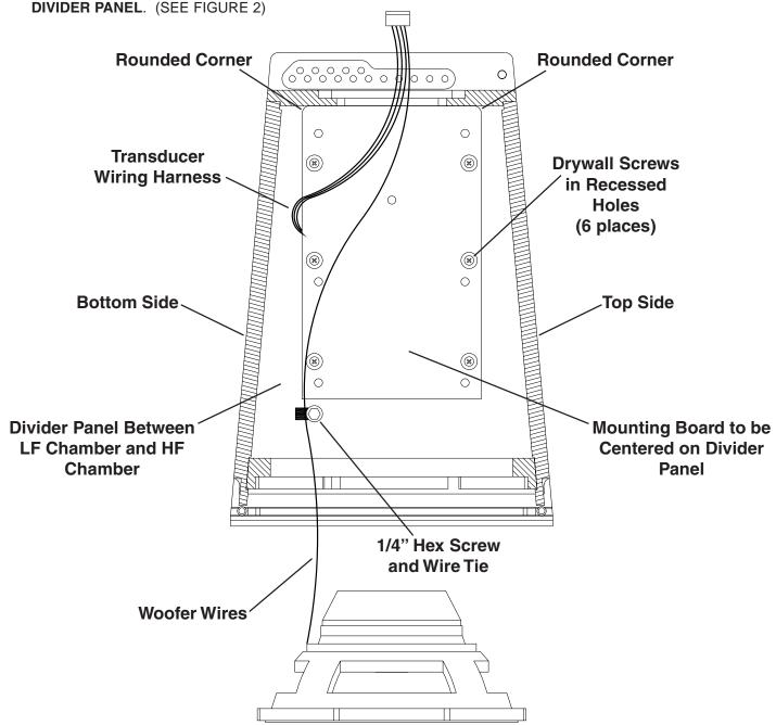
Figure 2: Attach Mounting Board to Divider Panel on Interior of Enclosure
