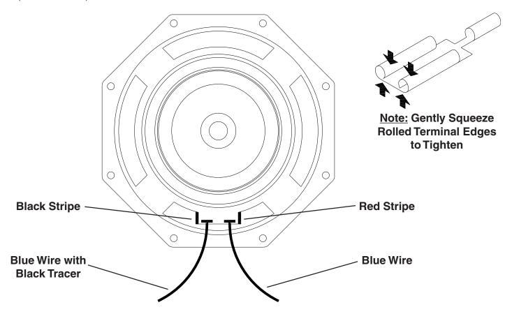
Figure 4: Re-Connect Woofer Wires to Terminals
