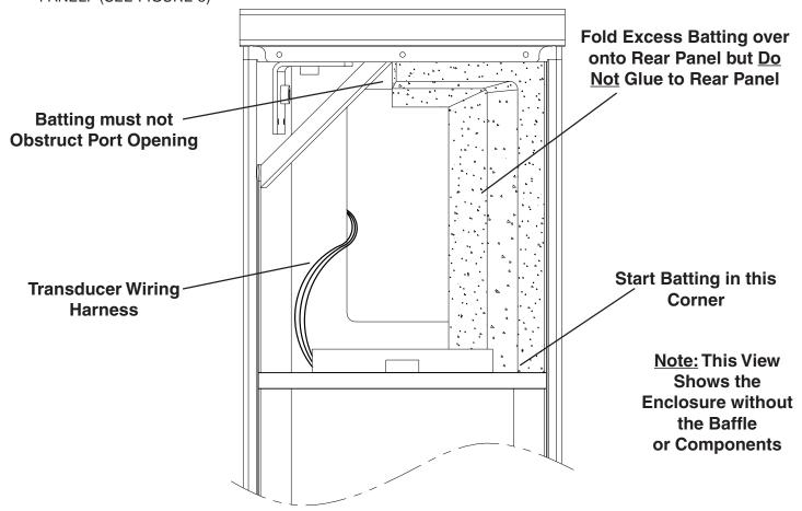
Figure 3: Installing New Batting in Low-Frequency Chamber
