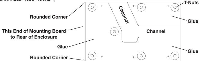
Figure 1: Apply Glue to Mounting Board
