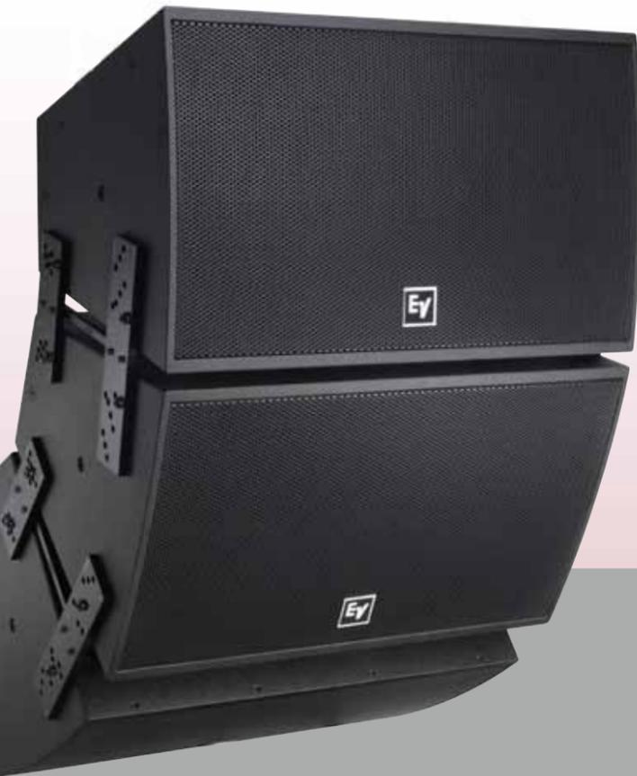
EVF systems have 22 or more internal rigging points, providing multiple choices for rigging the enclosures. Enclosures may be connected one above another using the supplied EBK-M10-EVI forged-eyebolt kits. However, commonly encountered clusters are more easily fabricated using the accessory HRK and VRK rigging kits. The rigging system is designed to carry a variety of array configurations in vertical or horizontal cluster formats with a safety factor of greater than 8:1.
